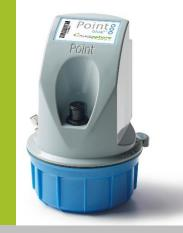
Point Blue IoT is an intrinsically safe, ATEX and IECEx certified compact Logger/RTU with a multi-band modem supporting NB-IoT and Cat-M1 networks, internal and/or external antenna, flexible I/O options, Modbus and SDI-12 master capability and a submersion sensor.
